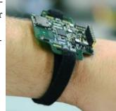
Using the PULPino processor, we are developing a smart watch equipped with electronics and a micro-camera. It can analyze visual information and use it to determine the user's whereabouts. The idea is that such a smart watch could one day control something like home electronics."
