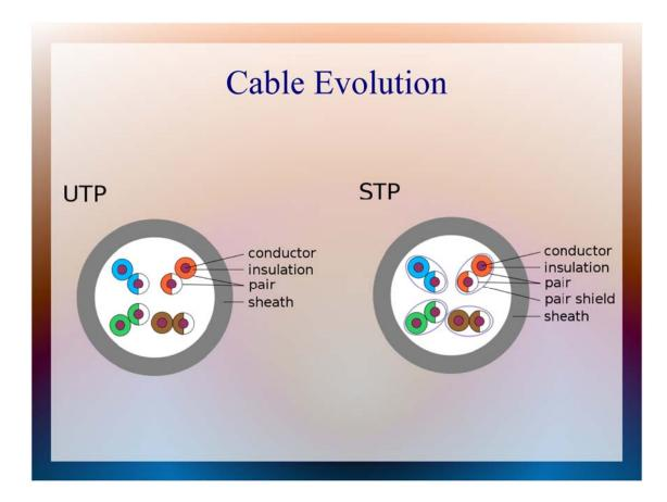
Unshielded twisted pair Shielded twisted pair To avoid Electomagnetic Interference
