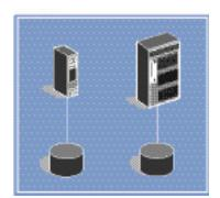
DAS: Direct Attached Storage. Storage (usually disk or tape) is directly attached by a cable to the computer processor. (The hard disk drive inside a PC or a tape drive attached to a single server are simple types of DAS.) I/O requests (also called protocols or commands) access devices directly.
