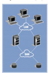
A SAN is a dedicated network for storage devices and the processors that access those devices. SANs today are usually built using Fibre Channel technology, but the concept of a SAN is independent of the underlying type of network.
