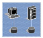
**Direct attach**—a single storage device is connected to a single processor (host).
