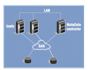
SANergy: SANergy is software from IBM and Tivoli that provides NASlike file sharing, with data sent over the SAN rather than the LAN for improved performance. (IBM NAS gateways also include SANergy function.)
