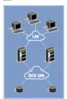
iSCSI is a proposed industry-standard that allows SCSI I/O commands to be sent over a network using the popular TCP/IP protocol. This is analogous to the way SCSI commands are already mapped to Fibre Channel, parallel SCSI, and SSA media. The proposal was made to the IETF (Internet Engineering Task Force) standards body jointly by Cisco Systems, Inc. and IBM, and is expected to be ratified in mid 2001. The iSCSI standard is also supported by SNIA (Storage Networking Industry Association).
