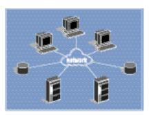
Network attach—one or more processors are connected to one or more storage devices.
