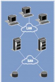
SAN: Storage Area Network. Storage resides on a dedicated network. Like DAS, I/O requests access devices directly. Today, most SANs use Fibre Channel media, providing an any-to-any connection for processors and storage on that network. Ethernet media using an I/O protocol called iSCSI is emerging in 2001.
