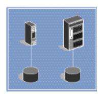
Direct Attached Storage is storage that is generally restricted to access by a single host (processor); sometimes by two hosts in small cluster (failover or failback) configurations. Even an enterprise-class disk system such as an IBM Enterprise Storage Server™ (ESS) can be effectively configured as DAS by assigning portions (partitions) of the internal disk capacity to
